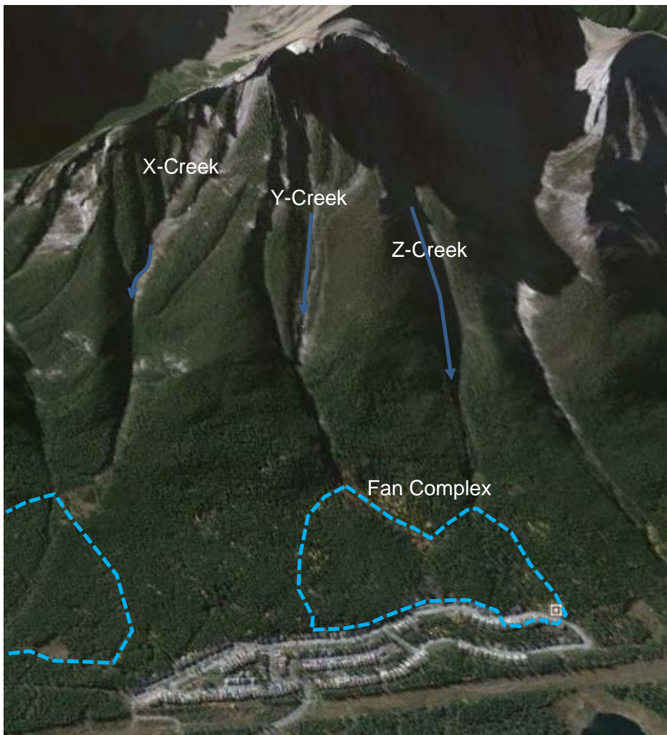
Figure 1-1. Google Earth satellite image of fan complex of X, Y and Z Creeks above the Grassi Peaks subdivision. The fan boundaries are approximate and require field verification.
