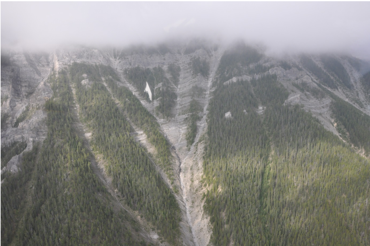
Photo 3-1. Overview of X Creek watershed showing a dendritic channel network characterized by a high frequency of snow avalanches that will likely displace much of the loose debris to lower watershed elevations. This watershed has a high runoff coefficient and will thus convey stormwater rapidly into the lower channel system where it may evolve into a debris flow. BGC photograph of July 23, 2013.
