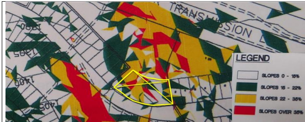
Slope plan showing proposed UR plot in yellow outline and slopes over 35% and slopes 22 - 35% associated with the rock outcrop (Source: Peaks of Grassi Phase III Land Use Report in support of an application for Amendment to the Land Use Bylaw. April 1998)
